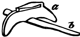
FIG. 36.—The " Ani-ani ," or Reaping Implement of Java. a , Hand-piece; b , Long Spatula, shaped left-hand piece.
